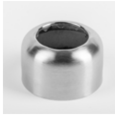
1-1/2 INCH I.P.S BOX FLANGE. 1-7/8 in. I.D. X 3 in. O.D. X 1-11/16 in. HT. Solid Brass Construction
