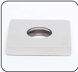
1/2 INCH SQUARE SHOWER ARM FLANGE. 13/16 in. I.D. X 2-1/16 in. O.D. X 9/32 in. HT. Held In Position By O-Ring Solid Brass Construction
