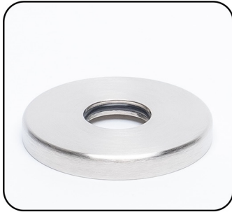
1/2 INCH SHOWER ARM FLANGE. 13/16 in. I.D. X 2-3/8 in. O.D. X 1/4 in. HT. Held In Position By O-Ring Solid Brass Construction
