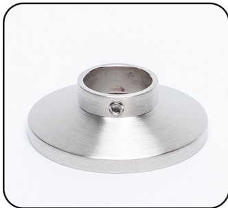
1/2 INCH SHOWER ARM FLANGE. 13/16 in. I.D. X 2-3/16 in. O.D. X 11/16 in. HT. Held In Position By Set Screw Solid Brass Construction
