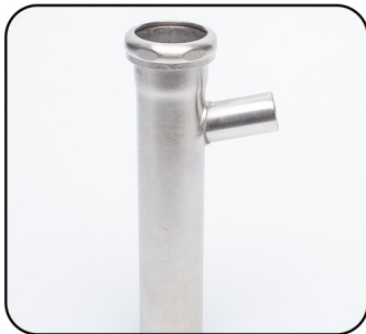
1-1/4 INCH O.D. X 8 INCH Y-BRANCH SLIP JOINT EXTENSION TUBE. 7/8 inch O.D. (3/4 inch Copper) Y-Branch Inlet Brass Nut 17-Gauge Solid Brass Construction
