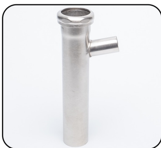
1-1/4 INCH O.D. X 8 INCH Y-BRANCH SLIP JOINT EXTENSION TUBE. 7/8 inch O.D. (3/4 inch Copper) Y-Branch Inlet Brass Nut 17-Gauge Brass Solid Brass Construction
